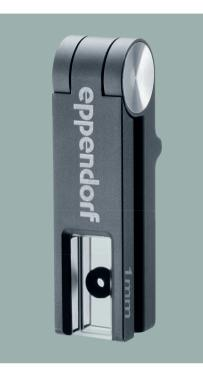
With an optical path length of only 1 mm, the  $\mu$ Cuvette G1.0 features a light path that is ten times shorter than the light path on standard cuvettes. This allows high nucleic acid and protein concentrations to be measured using the  $\mu$ Cuvette G1.0. Only 1.5  $\mu$ L of a sample is required for the measurement. The  $\mu$ Cuvette G1.0 offers a flexible expansion of the photometric application range of Eppendorf photometers.
