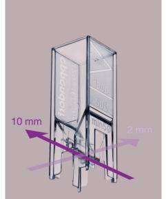
The patented\* Eppendorf UVette is a fully UV-transparent, single use cuvette made of clear plastic, with a light transmission of 220 nm to 1,600 nm. The unique design allows you to conduct flexible measurements with two different light paths (10 mm and 2 mm).
